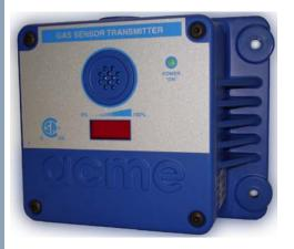
he Acme GasPost II toxic gas sensor/transmitter measures CO and NO2 gas concentrations in enclosed areas and transmits its readings to a CEL-series monitor/controller over an addressable RS-485 "Daisy-Chain" sensor network.
